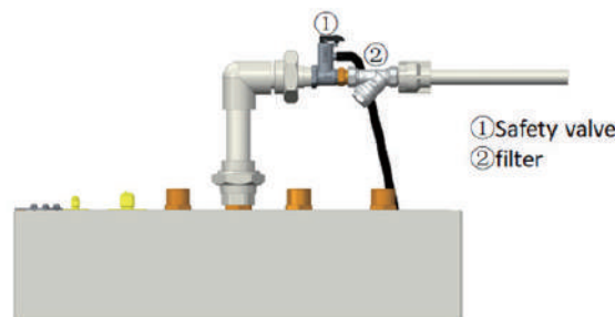
Installation Mode 1 of the Tap Water Safety Valve (Inlet Water Pressure =0.1~0.5MPa)
